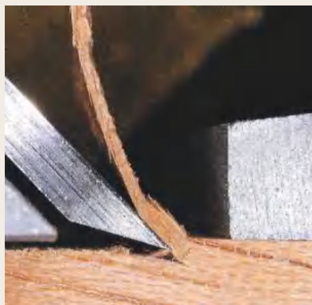
▲ Pic.3 Here I'm planing against the grain without a cap iron; note the stress marks at the root of the shaving
